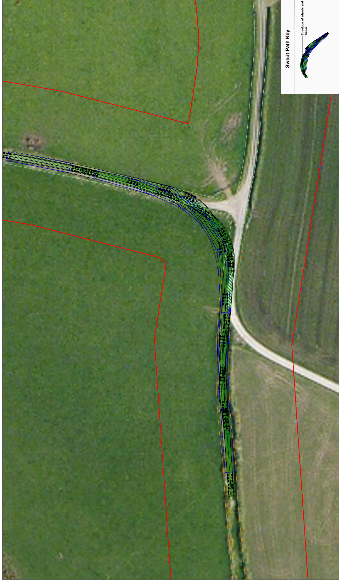
Figure 11.32 Location 13 - Right turn at Barnadvane, tower extended artic
