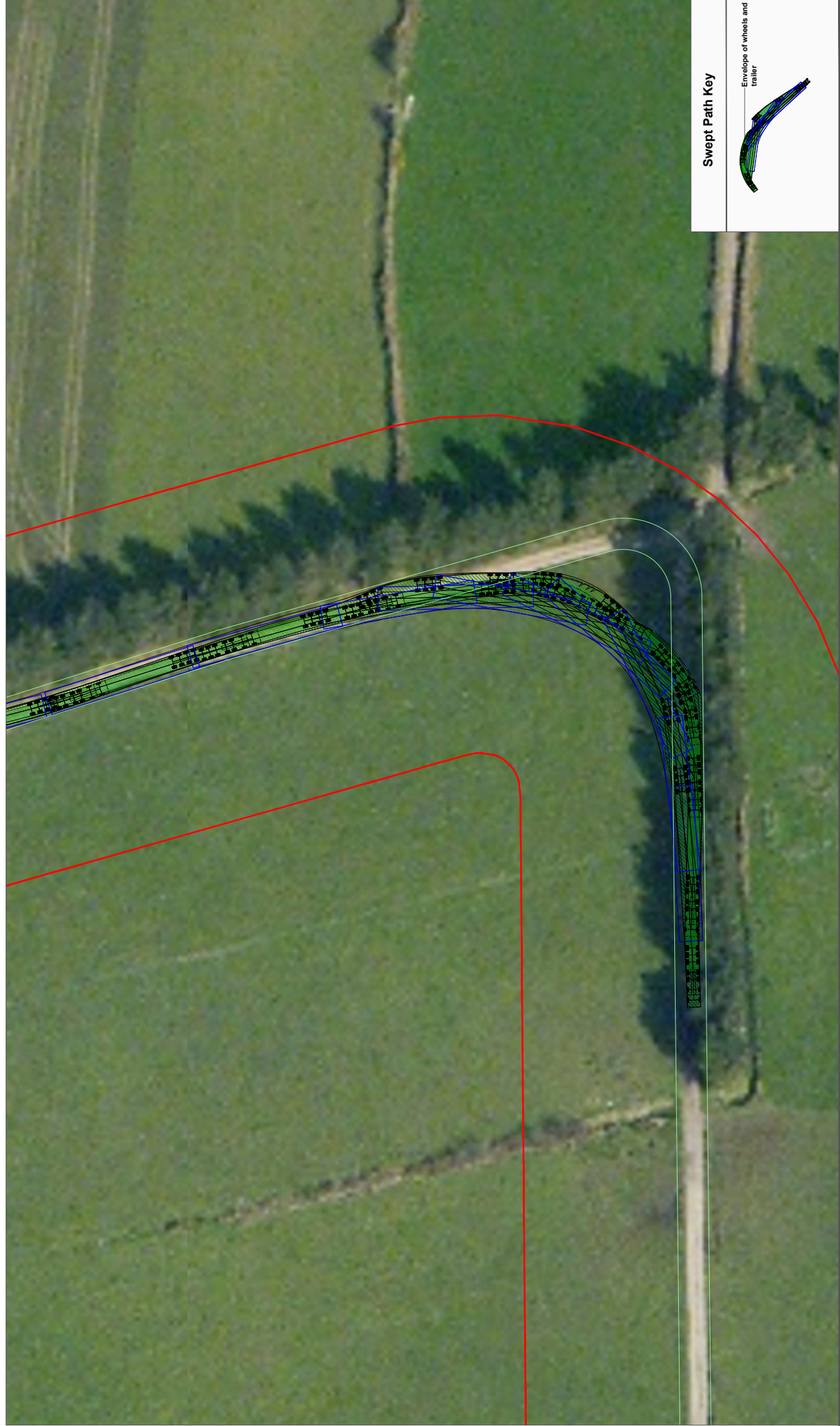
Figure 11.28 Location 11 - Right turn at Barnadvane, tower extended artic
